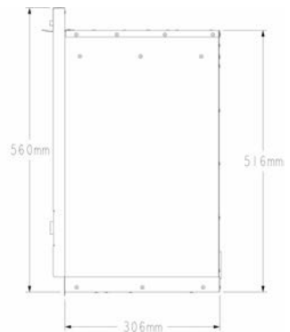
Side View of Combustion Chamber
