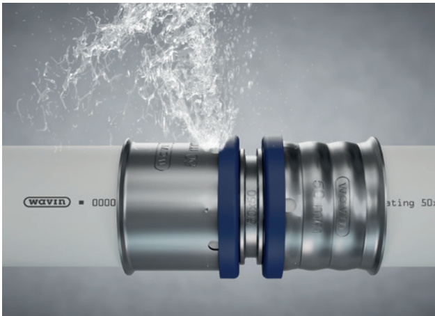
Fig.14: DEFINED LEAK in the pressure test reveals with leaking water the unpressed fitting.
