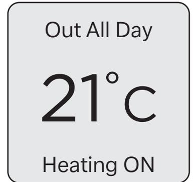
When the controller buttons have not been pressed for a long period of time, the display will 'sleep' and the text will disappear. The heater is still on and active in whatever Mode it was set to.
