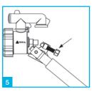
The water level can be adjusted by turning the adjustment screw (clockwise for less water, anticlockwise for more water)
