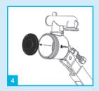
Remove the diaphragm washer and clean or replace.
