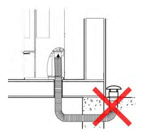
If the air intake is turned upwards, there will be too much resistance for the air intake.
