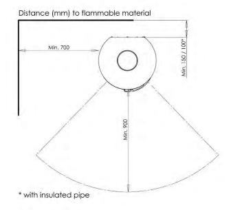
If the stove is positioned against a brick wall or other non-flammable material, there are no minimum distance requirements. To facilitate cleaning and for the best use of the convection air, we recommend that you leave a distance of approximately 5-10 cm to the wall.
