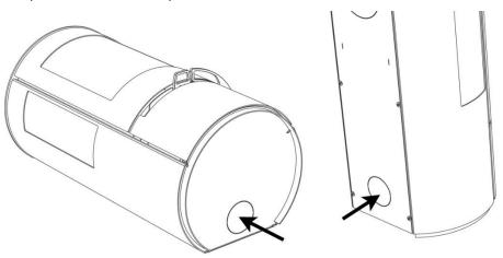
If you want to use the wood burning stove without connecting the supply of combustion air, "brake" off the cover plate in the rear cover at the bottom of the back of the stove.
