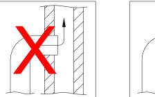
The wood burning stove can be connected to a chimney to which other heat sources are connected.
