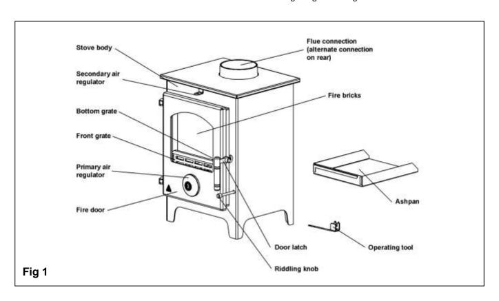
The highest burning rate is achieved by opening the air regulator wheel to maximum. Excess ash formation may indicate over firing.
