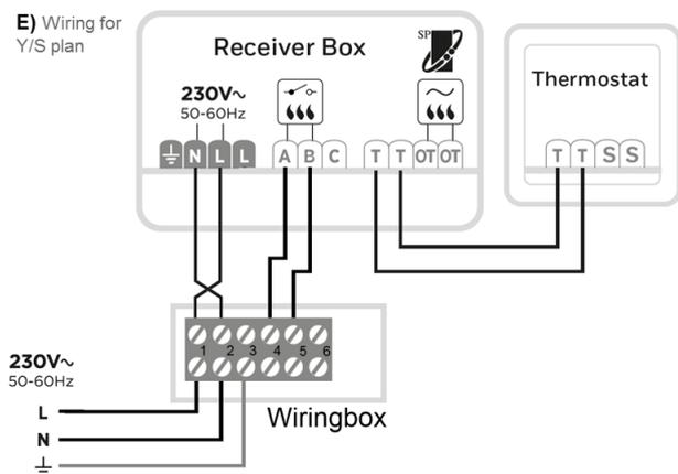
Note: Wiring diagrams are for T6 wired thermostat solution, for T6R wireless thermostat the thermostat is not wired to the Receiver box and the terminals are also not available.
