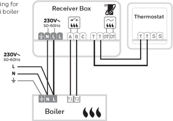
**C)** Wiring for OpenTherm boiler
