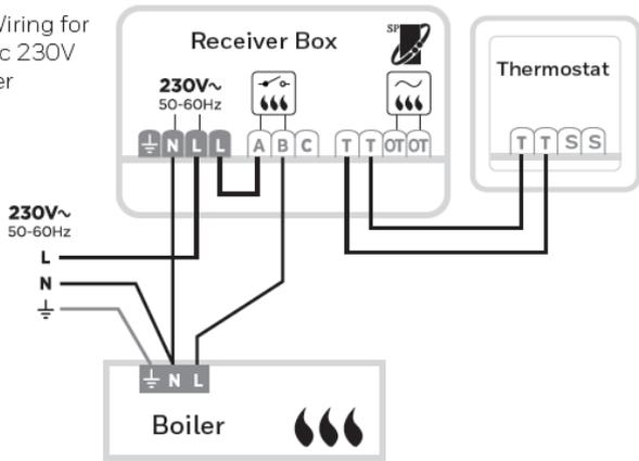
**B)** Wiring for Combi boiler
