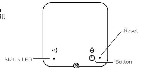
2. Enable binding on the thermostat:
