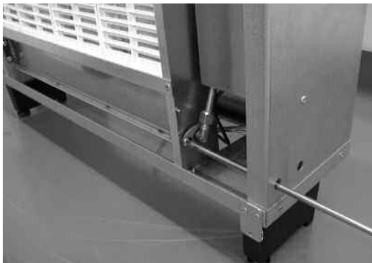
Fig. 11 Injector fixing bracket removal
